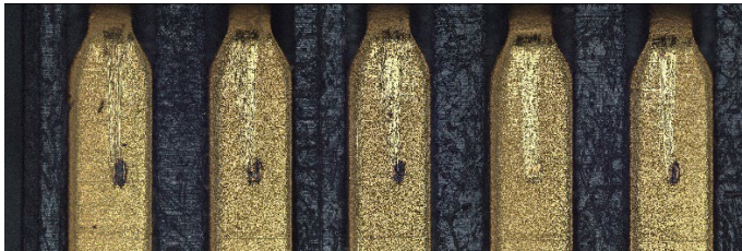
Fig.1: Example gold plated electrical contacts exhibiting connector wear after a vibration test
