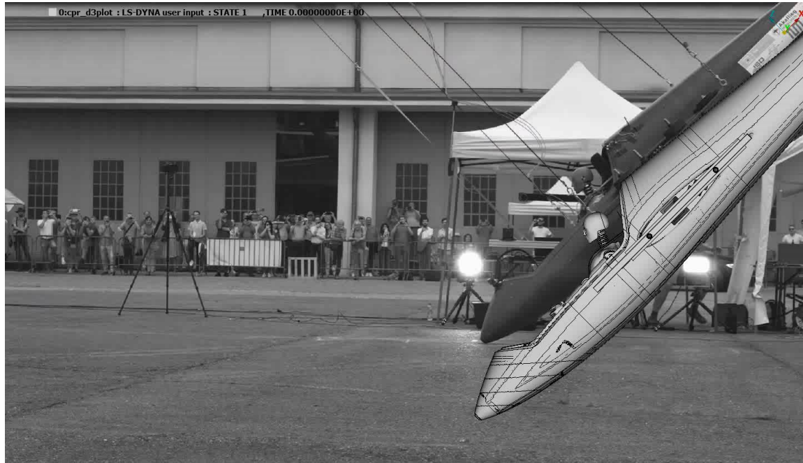
Fig. 19: Side view of crash test vs simulation
