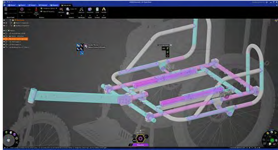
Structural analysis of Advenchair assembly within Ansys Discovery. Courtesy on Onward Project LLC
