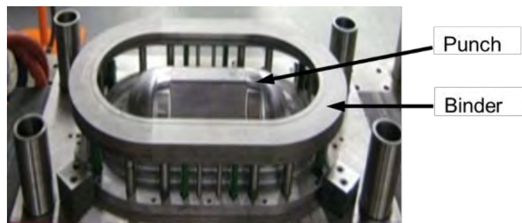
Fig 2: Experiment setup for the double dome test.
