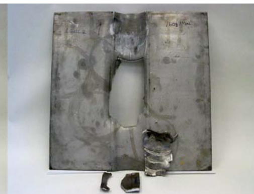
Figure 11 Curved Plate at 1600 ft/sec
