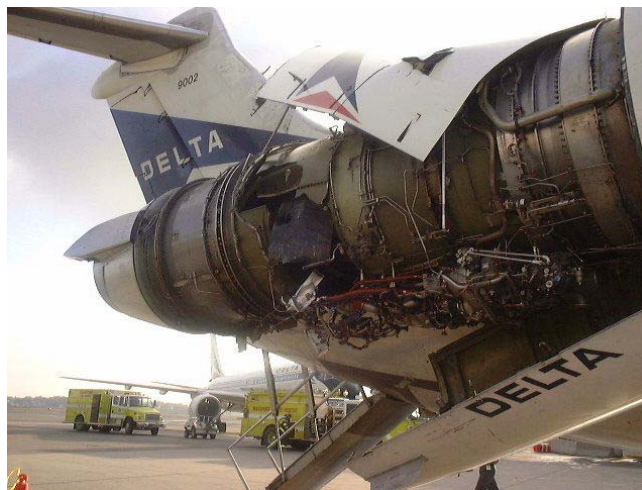
Figure 1 Uncontained Engine Failure
