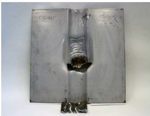
Figure 10 Curved Plate at 1500 ft/sec
