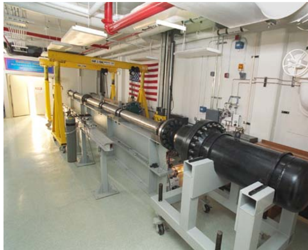
Figure 3 Glenn Research Center Ballistic Impact Laboratory Gas Gun
