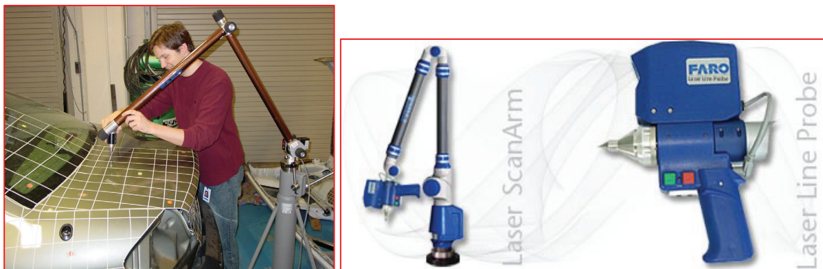
Fig. 3: a) 6 DOF Coordinate Measuring Machine b) Laser Scanner
