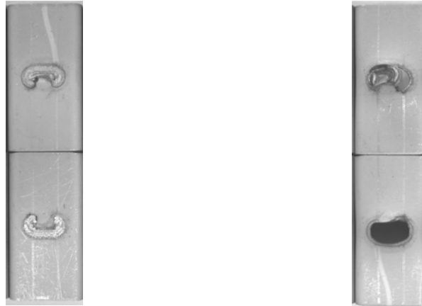
“Weld tear off” in a KS2 0° 1.5mm-1.5mm gauge combination
