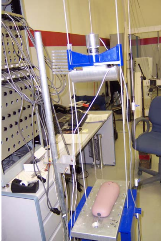
Arm drop test set-up
