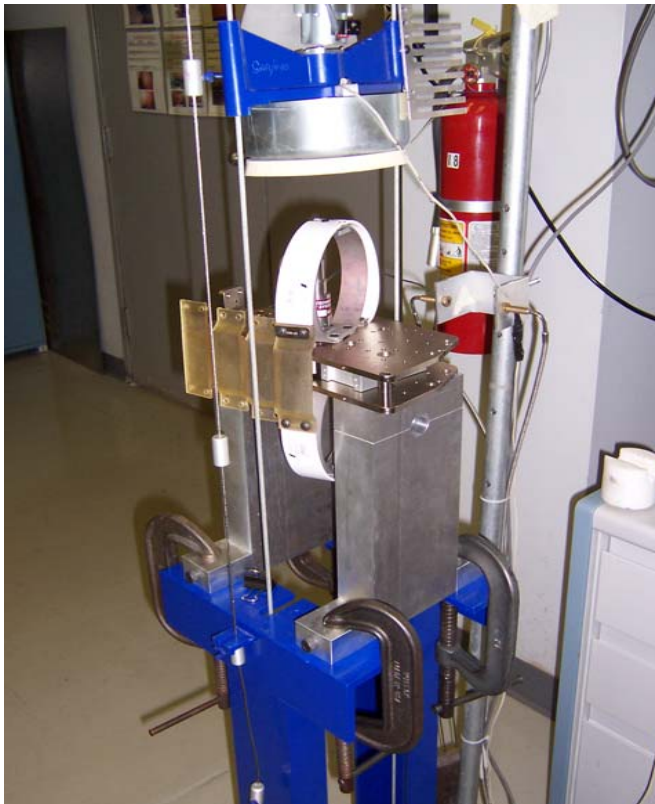
World SID 5 th rib drop test set-up
