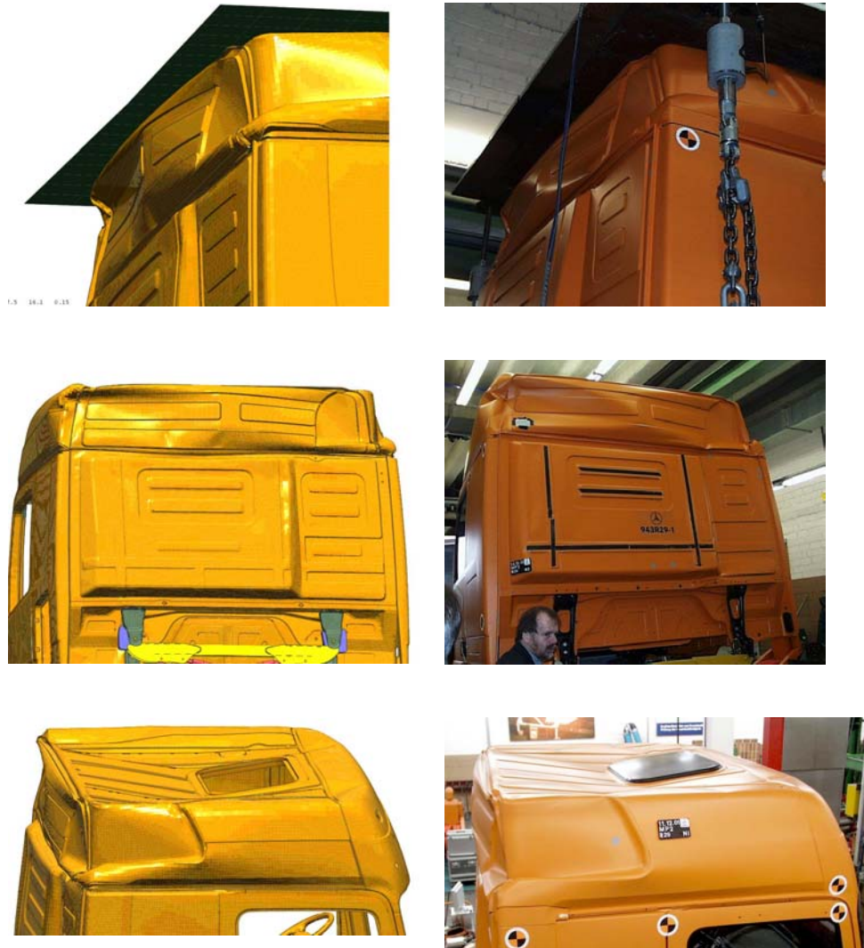
Fig. 13: Comparison of Roof Deformation Resulting from Numerical Simulation and Acceptance Test
