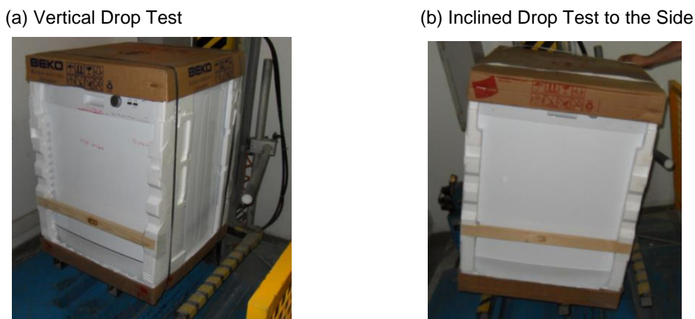
Fig. 2: Experimental setup a) Vertical drop test b) Inclined drop test to the side
