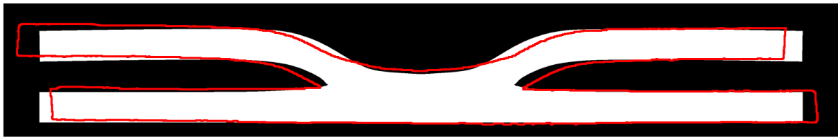
Fig.13: Comparison between the cross-sections of the numerical result (white) and the experimental result (red line).
