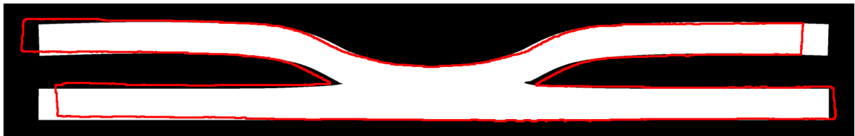
Fig.14: Comparison between the cross-sections of the numerical result with increased strain rate sensitivity (white) and the experimental result (red line).
