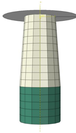
Fig.3: FE model of the micro-pillar (originally from Prof. Farhang Pourboghrat, MSU) used in the CP calibration. The lower part (dark green) represents an elastic foundation. The base is constrained at the bottom and a downward compressive force is applied at the top.
