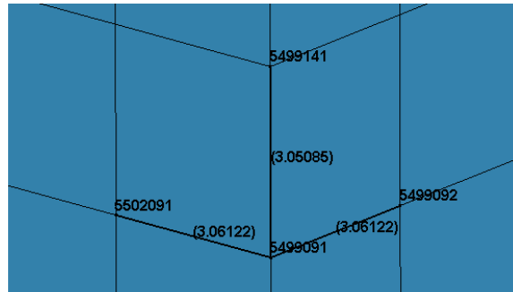
Figure 5. Characteristic Element for Parametric Simulations (3.05 cm X 3.06 cm x 3.06 cm)
