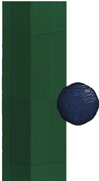
Figure 7. 42-in. Square Column, 100-lb TNT, 40.8-in. Standoff: (a) 114 usec; (b) 258 usec [315]
